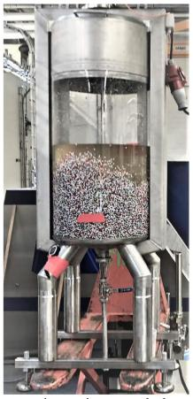
Tetra Pak delivers liquid food processing equipment and a key component in almost all processing lines are tanks. Tetra Pak operates several types of tanks such as buffer tanks, mixing tanks and aseptic tanks. Here we will focus on a 200L vertical tank with a purpose to keep a homogeneous mixture.
