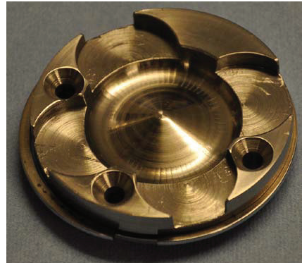
Figure 1. Installed piston crown
