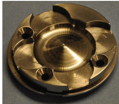
Figure 1. Installed piston crown.
