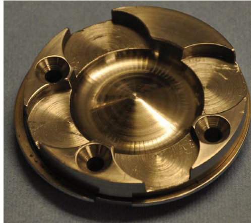
Figure 4 - Photograph of the modified piston with valve pockets.
